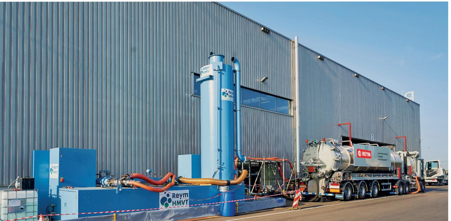
Some vapors released during industrial cleaning operations cannot simply be released into the atmosphere. REYM-HMVT has a wide range of flexible, mobile treatment plants to effectively clean these vapors. Vapor cleaning is an integral part of the cleaning process and maintenance work.
