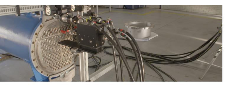
REYM uses an internally developed lance tube cleaner, the Evolvere, to clean pipes and bundles. With this machine, REYM adopts the advice of the Industrial Cleaning Foundation (SIR) to use (fully) automatic cleaning equipment as much as possible. The machine is operated remotely so that the employee is at a safe distance.
