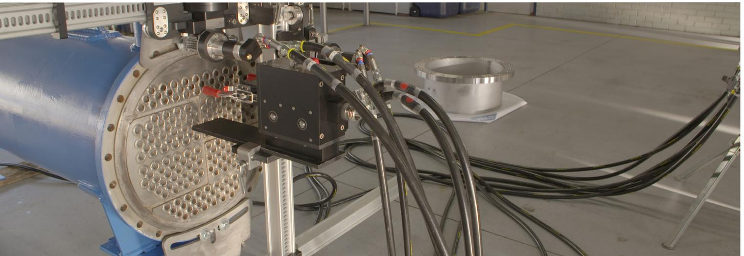
REYM uses an internally developed lance tube cleaner, the Evolvere, to clean pipes and bundles. With this machine, REYM adopts the advice of the Industrial Cleaning Foundation (SIR) to use (fully) automatic cleaning equipment as much as possible. The machine is operated remotely so that the employee is at a safe distance.
