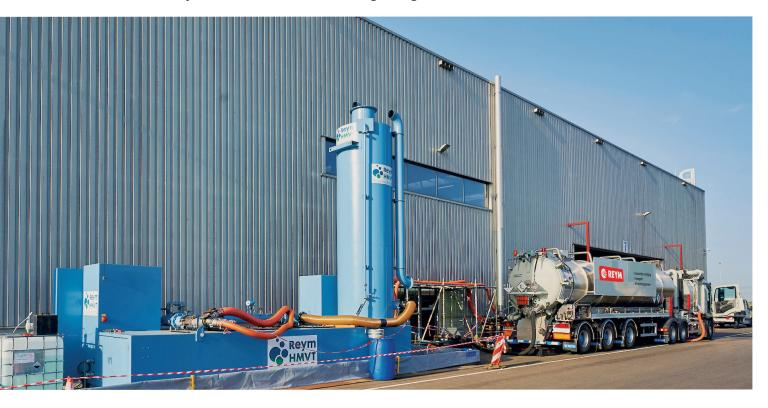
Some vapors released during industrial cleaning operations cannot simply be released into the atmosphere. REYM-HMVT has a wide range of flexible, mobile treatment plants to effectively clean these vapors. Vapor cleaning is an integral part of the cleaning process and maintenance work.
