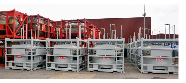
REYM has twelve T14 classified tanks with top inlet and discharge option. They can be used for specialist cleaning assignments, offshore as well as onshore.
